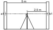
Set up the instrument 0,5-0,7m away from the wall and make, as described above, the same masrks. If the difference  $\{a1-b2\}$  and  $\{b1-b2\}$  is less then the value of "accuracy" (see spesifications), there is no need in calibration.
